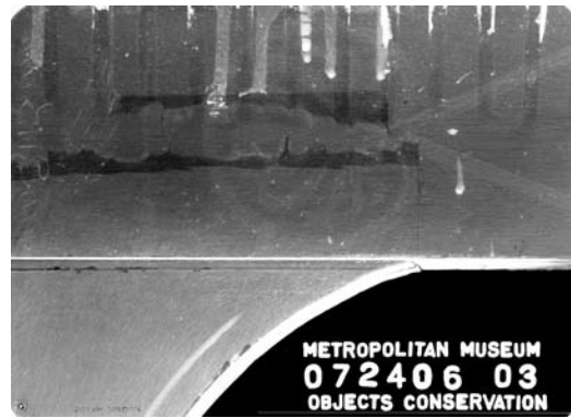
Figure 3 X-radiograph of the joints of the proper right seat rail with the rear stile and rear leg. Note the rough-cut mortises and the paint drips on the inside of the seat rails.
